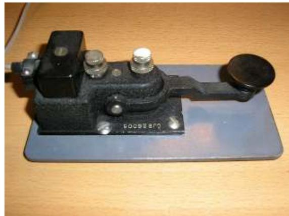
This key is called "flame-proof" because the contacts are within the body of the key and would not ignite any explosive vapors in the immediate area of the key.
