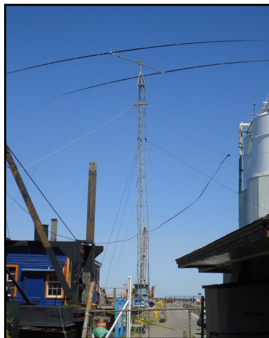
2L 20m yagi mounted on 28 ft tower at the K8O site. Antenna was fixed south-west
