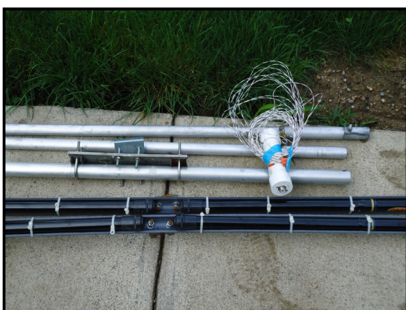
The entire 2L 20m yagi; balun, wire elements boom and crappie poles
