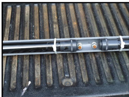
Mounting of the crappie poles to the pvc sections and the muf-fler clamp that will hold the elements to the boom. That pile is the entire antenna.
