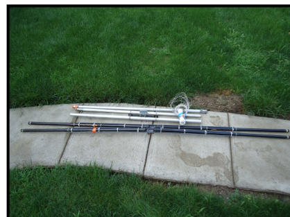
Mounting of the crappie poles to the pvc sections and the muf-fler clamp that will hold the elements to the boom. That pile is the entire antenna.
