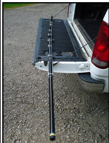
Mounting of the crappie poles to the pvc sections and the muf-fler clamp that will hold the elements to the boom. That pile is the entire antenna.
