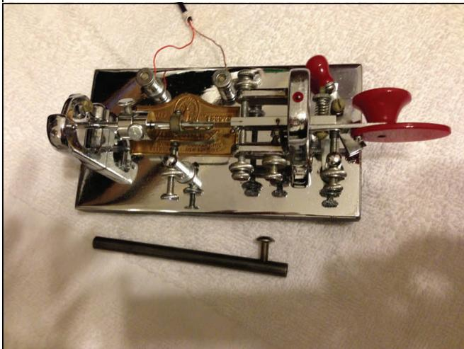
Here is the bug in position with the “speed control” installed.
