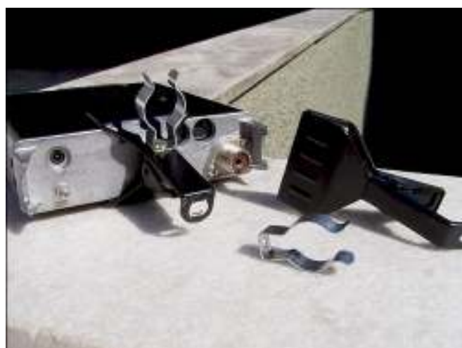
Security camera mounting clamp for securing the radio
