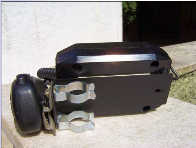
Loudspeaker and microphone. Notice the fluorescent light clamps
